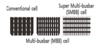
Multi-busbar - reduced strings increase output, dense wires reduce losses
