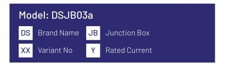
• DSJB03a - Rated current 15A & screwless-type clamping for pv ribbon
