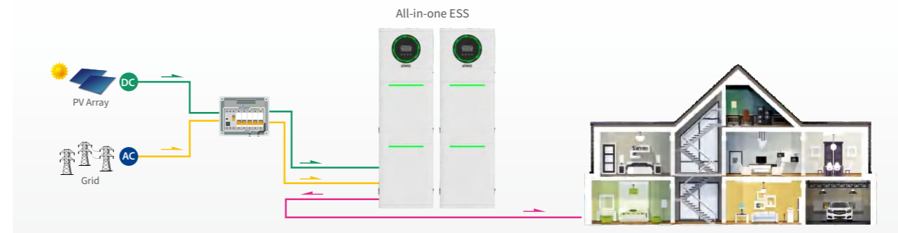
Three phase 18kw Inverter with 30720Wh Lithium Battery
