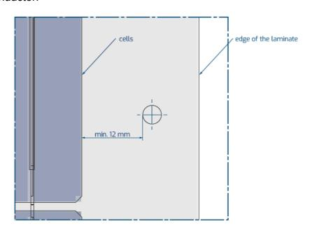
The edges of the cut holes <u>should be sealed</u> to prevent moisture from entering the fibre reinforced composite material. A suitable sealant for outdoor applications can be used. Note that inadequately sealed cut or drilled surfaces will void the warranty.
